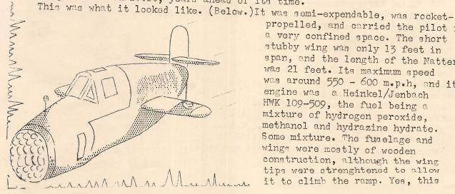
propelled, and carried the pilot in a very confined space. The short stubby wing was only 13 feet in span, and the length of the Natter was 21 feet. Its maximum speed was around 550 - 600 m.p.h, and its engine was a Heinkel/Jenbach HWK 109-509, the fuel being a mixture of hydrogen peroxide, methanol and hydrazine hydrate. Some mixture. The fuselage and wings were mostly of wooden construction, although the wing tips were strenghtened to allow it to climb the ramp. Yes, this
